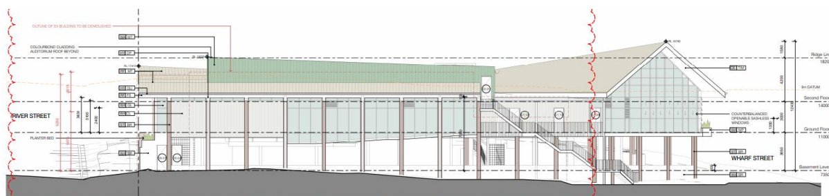
Figure 15: The North Elevation, being the low point on the site, shows the greatest variation from the standard. The 9 m datum line is shown as an orange dashed line, with the existing roof line shown as a red dashed line.
